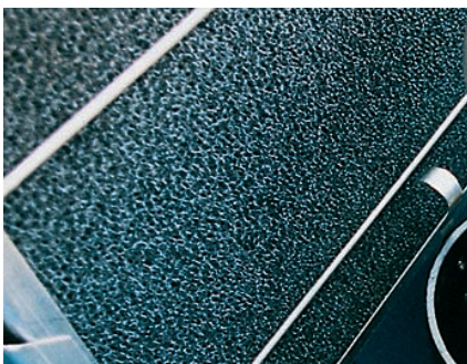
Image 2a: Coalescence insert made of PU
